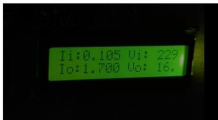
Notification through buzzer at set threshold (1.70 Amp)
