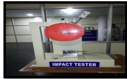
Figure 22 Impact machine for impact testing
