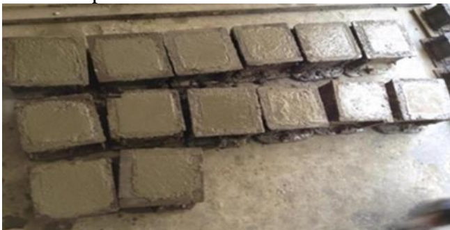
Fig.2.4: Mixing and casting of fresh concrete
