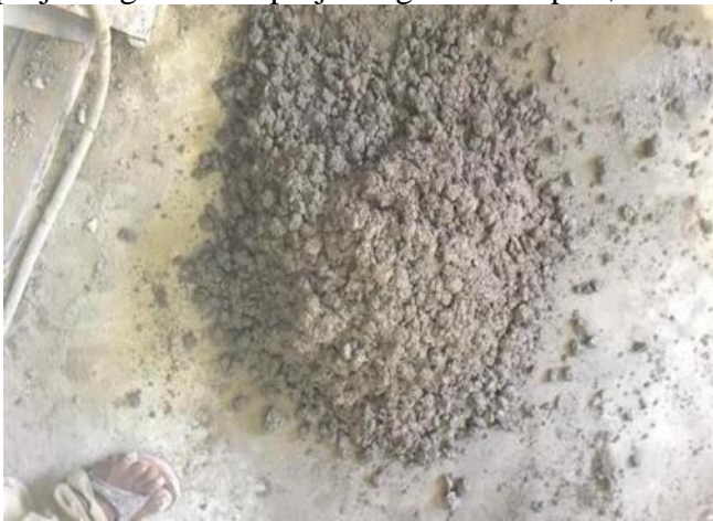
Fig.2.3: Mixing of Recycled aggregate concrete
