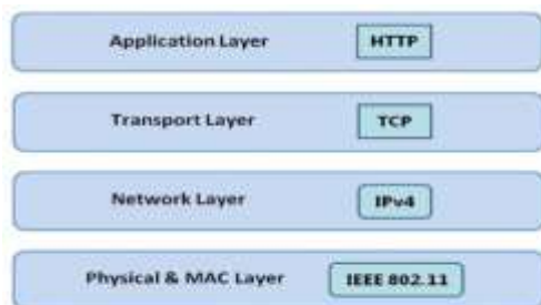
Fig. 17. ESP8266 communication layers and protocols.
